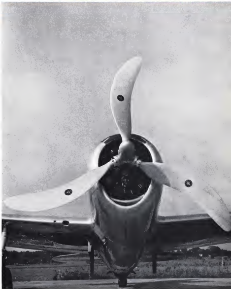
Curtiss' Swept-Back Blades: In an attempt to push blade speeds into the transonic range, Curtiss-Wright Corp. has developed this swept-back propeller for AAF. With it, the manufacturer claims propeller-driven aircraft can attain speeds perhaps as high as 700 mph. The propeller is mounted on a Republic P-47, indicating it is designed to absorb approximately 2,000 hp. (Story on Page 10)
